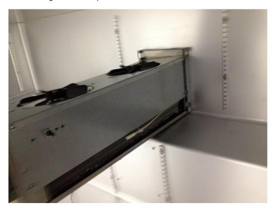
**9.** Install aluminum outer panels and top panel (hat). Replace knob on control. Re-attach the shelving brackets with the thumb screws.
